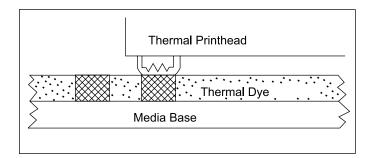
Direct thermal printing uses chemically treated, heat-sensitive media that blackens when it passes under the thermal printhead. Direct thermal printers have no ink, toner or ribbon. The simple design makes thermal printers durable and easy to use. Because there is no ribbon, direct thermal printers cost less to operate than thermal transfer models.
