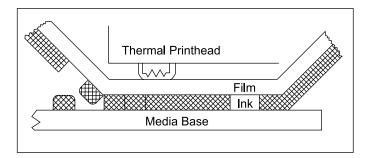
In thermal transfer printing, a thermal printhead applies heat to a ribbon, which melts onto the label material to form the image. The ribbon material is absorbed into the media so that the image becomes part of the label. This technique provides image quality and durability that is unmatched by other on-demand printing technologies.
